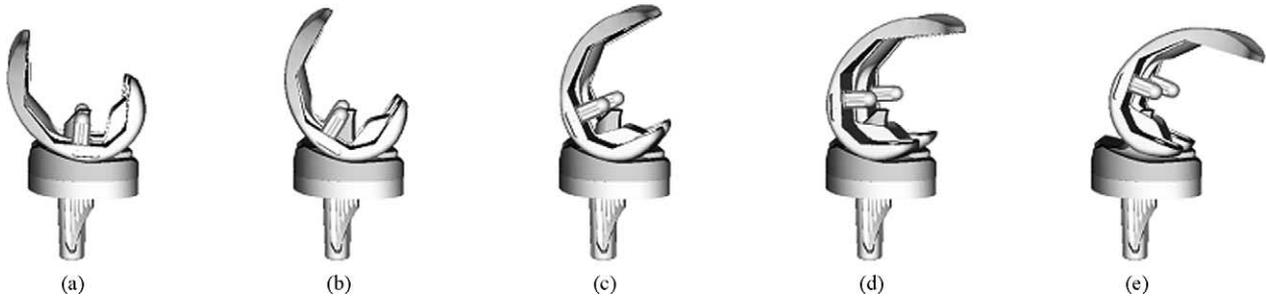
Fig. 5. Relative movement between the femoral component and the tibial component with the tibial insert. The movement is shown as the positional relationships at flexion angles of (a) 0.0°, (b) 31.9°, (c) 66.4°, (d) 87.8°, and (e) 110.7°.
