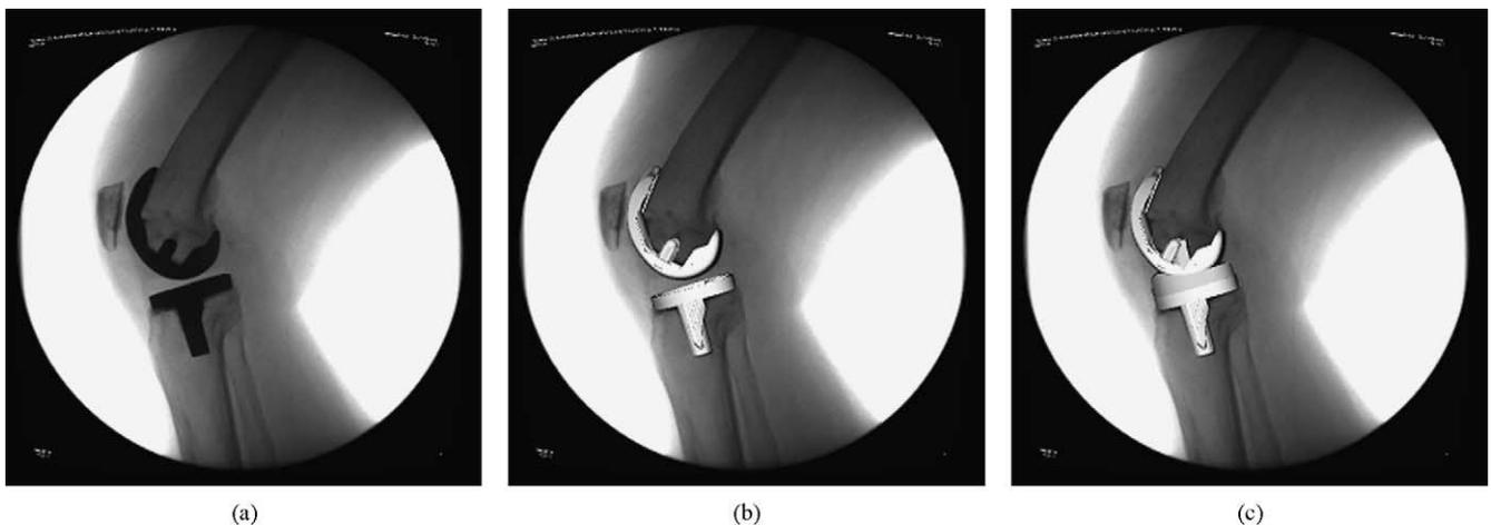
Fig. 4. X-ray and CAD model images from a TKA patient during deep knee flexion. (a) Representative X-ray fluoroscopic image. (b) Image with femoral and tibial CAD models overlaid. (c) Image of virtual tibial insert model between the femoral and tibial components.
