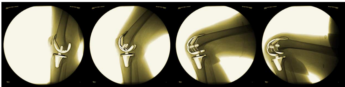
Fig. 2. Results for two- to three-dimensional registration overlaid on a sequence of fluoroscopic images during deep knee bending.
